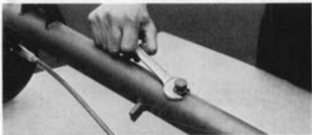
On the required side and near the centre front, slacken the locknut on the axle tube. Remove the cone screw and locknut.
