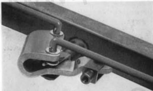
Correct setting of compensated brake linkage on square beam axles.
