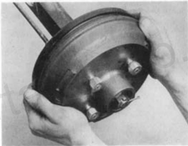
Check taper roller bearing adjustment by rocking hub. There should be little or no perceptible shake but should be complete freedom to rotate. (For lubrication of taper roller bearings see "Assembly of hubs fitted with taper roller bearings"). If excessive play is present new bearing assemblies must be fitted.
