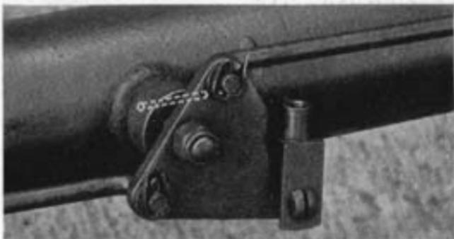
Correct setting of compensated brake linkage for torsion bar axle.
