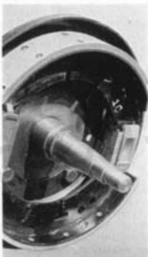
(d) The taper roller bearing cones must be greased (spec. as (b)) **ensuring that the grease penetrates inside the roller cage, between the rollers and the cones.**
