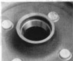
(c) The operating diameters of the axle must be clean.
