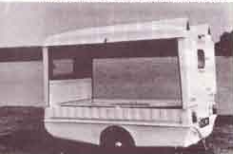
4. With the two ends and the roof locked together, you are now ready to lift the inner walls.
